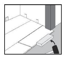
Step 1: Undercut space under door jamb to allow plank to slide freely. Tap long edge with hammer and tapping block to lock long edge of vinyl so as not to damage locking profile.
