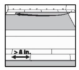
Step 3: Use leftover plank (min 8") from first row as starter for second row. There must be at least and 8" stagger between plank end joints on adjacent rows.
