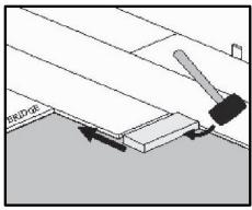
Step 7: Tap end of plank with hammer and tapping block to lock ends of planks together. Remove bridge and continue towards wall until installing the
